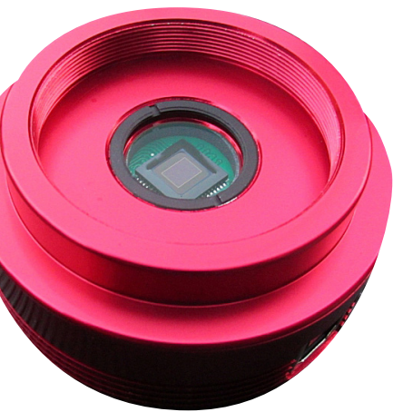
▲ The window over the CCD chip. Some early models are lacking the window, leading to dust build up on the chip.
