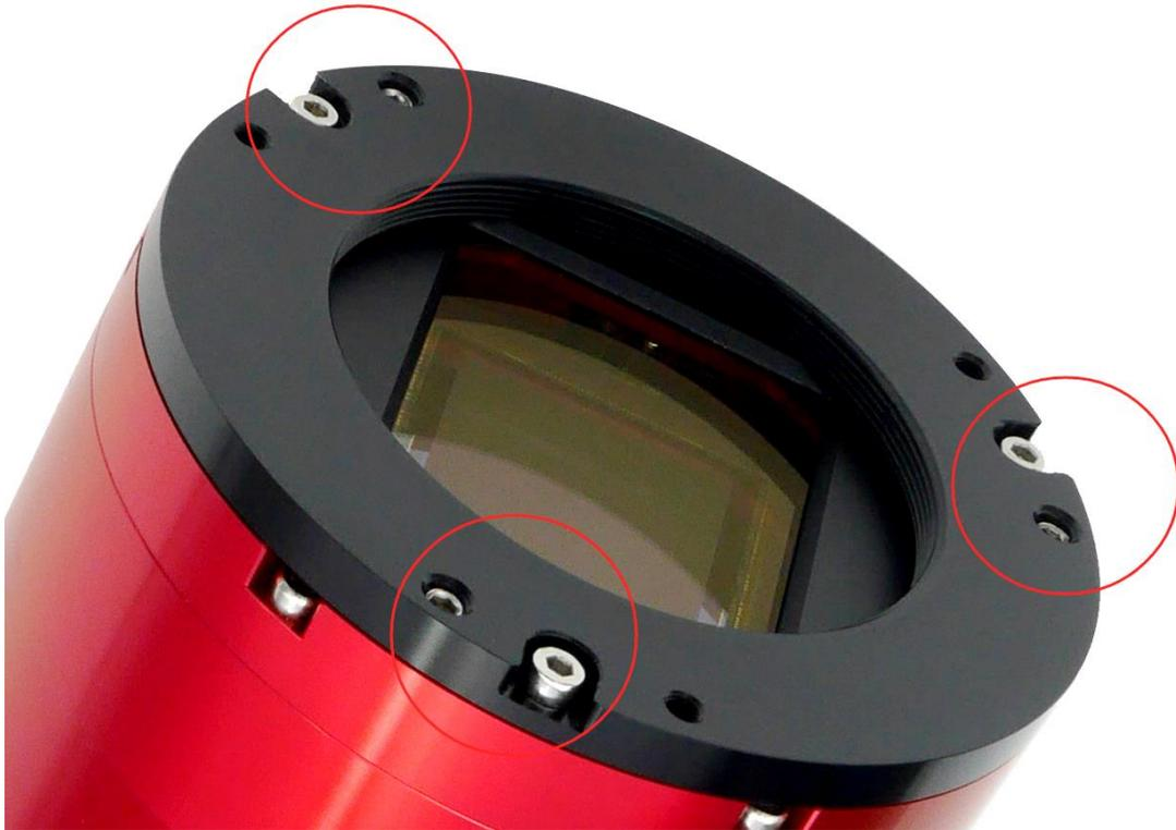
1. Find out which part of the camera has a tilt issue from your image and mark it on the camera body, then you can adjust the screws in this direction or opposite direction in the next step.
