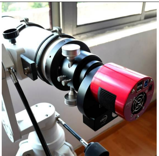
Install the T-mount to the back of the EFW.
