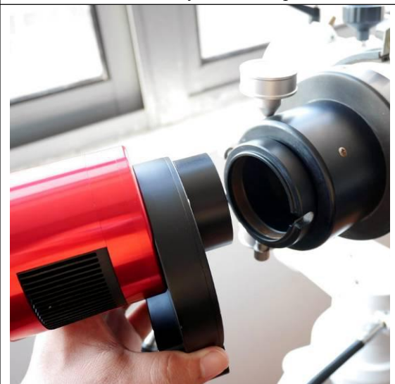
T2 extender can be used for attaching the telescope with 2" interface.
