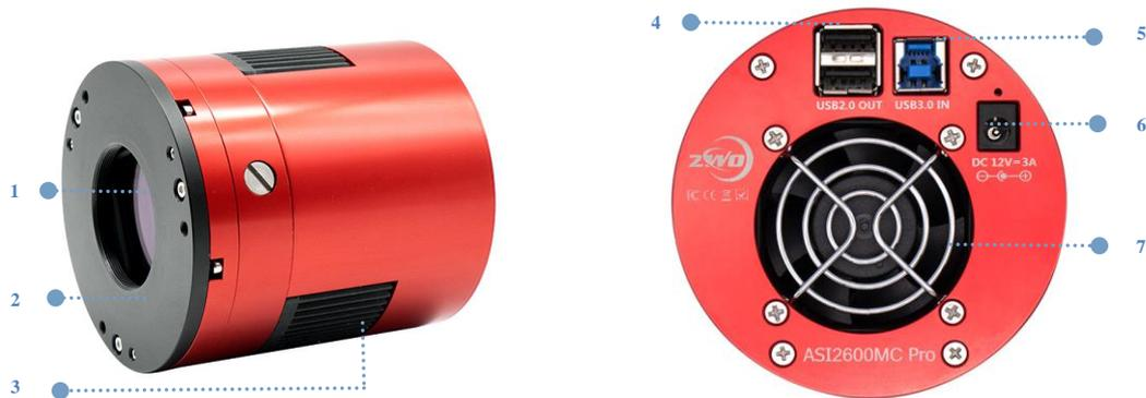
1. Protective Window, IR CUT, D60\*2mm
