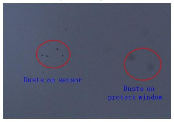
The big dim spot on the image (at right) are the shadows of dust on the protective window.
