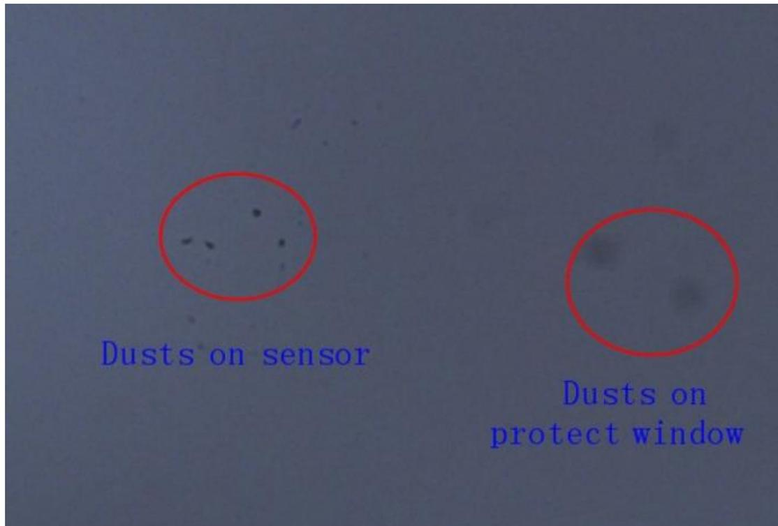
The big dim spot on the image (right side) are the shadows of dust on the protect window.
