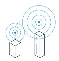
Wireless repeaters are first generation WiFi signal extenders. As the name implies, wireless repeaters re-broadcast the WiFi signal received to a finite localized area. The quality of WiFi signal strength received by the wireless repeater will be the same WiFi signal strength distributed. Latency, or WiFi network response time, is typically increased. If you need a short hop, have less than 5 wireless devices and are not going to stream anything, a repeater might work.
