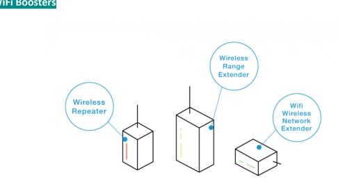
The term WiFi booster was a catch-all phrase for devices that extended a WiFi signal. A WiFi booster now is more accurately defined as a wireless range extender, wired extender or an Ethernet WiFi Wireless Network Extender.
