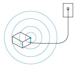
WiFi Network Extenders are the best WiFi boosters for consistent, reliable high speed WiFi to every floor and corner of your home. Unlike repeaters or range extenders that rebroadcast existing WiFi signals, WiFi Network Extenders communicate directly with your gateway or WiFi router using a wire.
