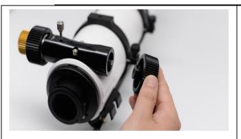
Remove the coarse adjustment knob of the telescope focuser using a suitable sized wrench
