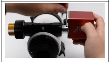
Attach the focuser body to the flexible coupler and tighten the lock screw using the supplied wrench
