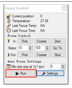
SGP will automatically take exposures and move the focuser steps drawing a V curve tracking the stars HFR value. Once the curve is complete SGP will drive the focuser to the best measured value.
