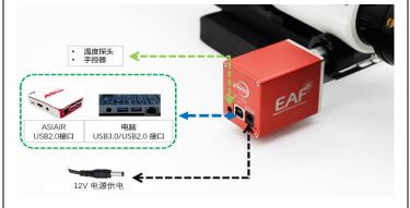
Connect the EAF to a 12V power supply and connect to the USB cable to a computer or ASIAIR.
