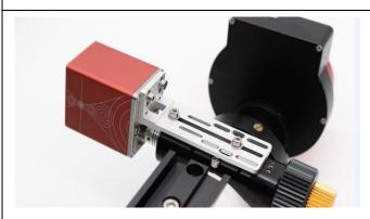
Check all the mounting bracket is secure. This completes the hardware installation of the EAF. Download and install the required drivers from the ZWO website as required.
