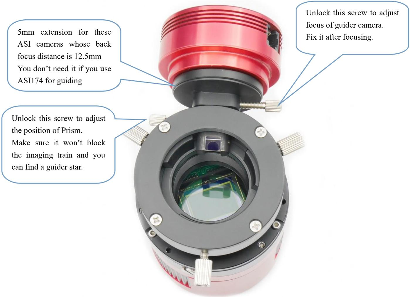
You'd better do it at day time to make sure imaging camera and guiding camera can reach focus together.
